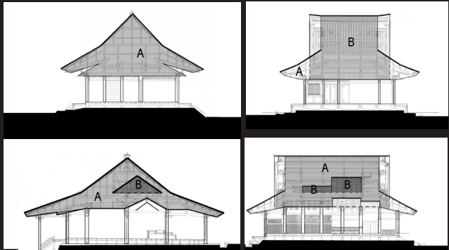
A=space created by intersecting roof geometries B=space created by hidden roof
